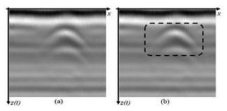
FIGURE 2: B-SCAN IMAGE CAPTURED FOR A CONCRETE OBJECT WHICH IS BURIED UNDER 3 CM
