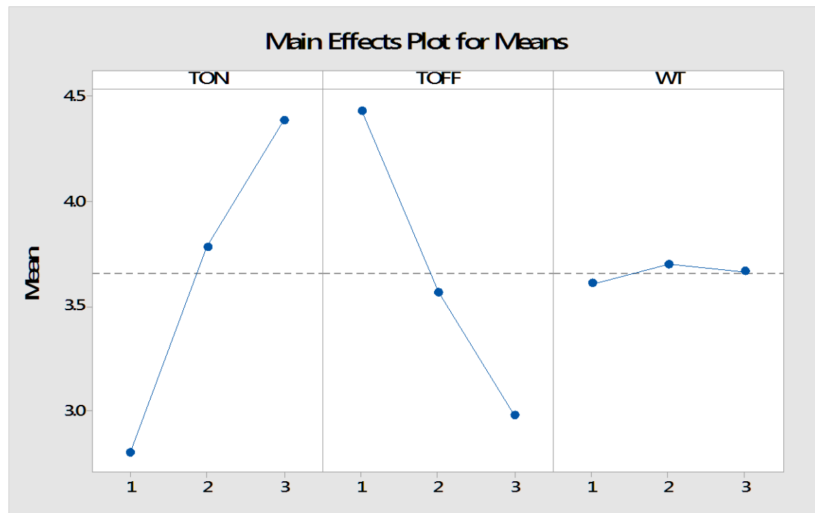
Fig 3.3.1.effect of process parameters on material removal rate (S/N Data)
