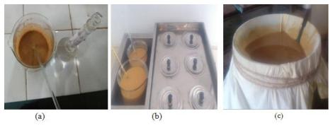
Fig 2 (a) Peel water mixture (b) Water bath heating (c) Filtration
