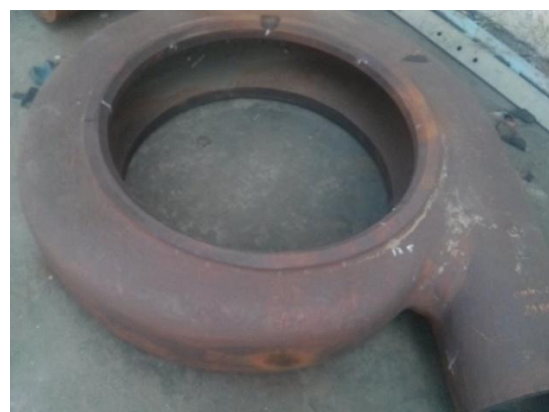
FIGURE 2- New Casing (Unused)
