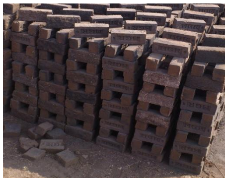
Fig.no.3.1.2. Drying of Bricks
