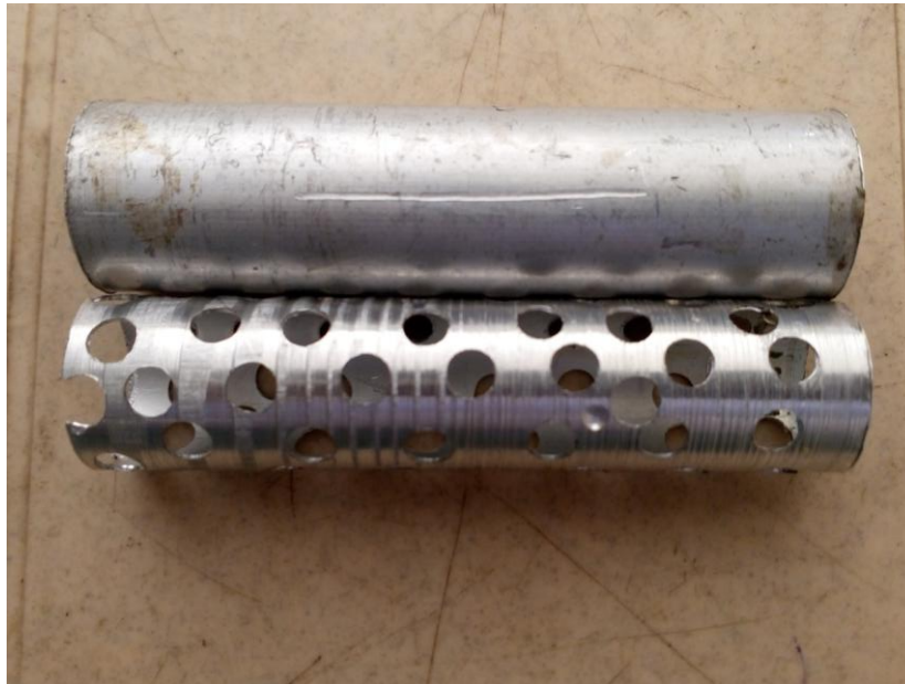
Fig. 10. Inner tube before and after drilling holes on surface
