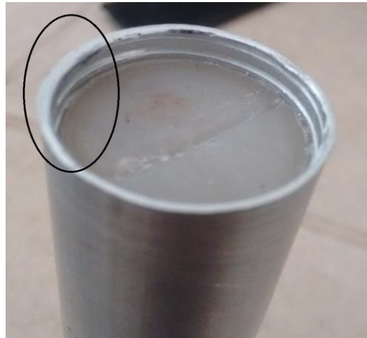
Fig.8. Shrinkage After cooling.
