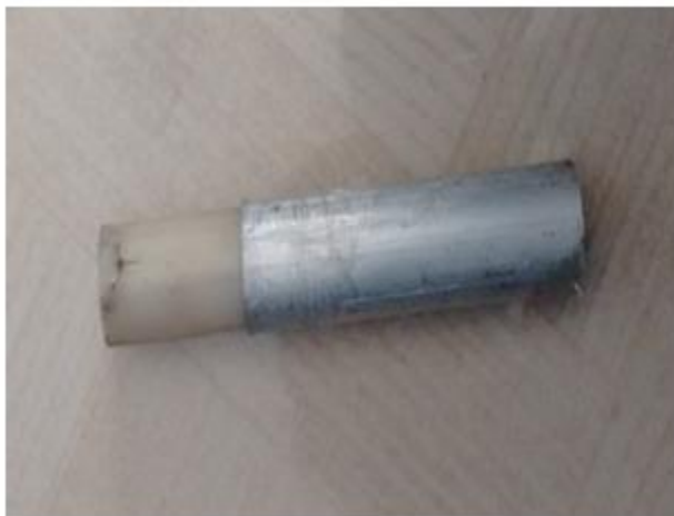
Fig.5. Debonding due to shrinkage
