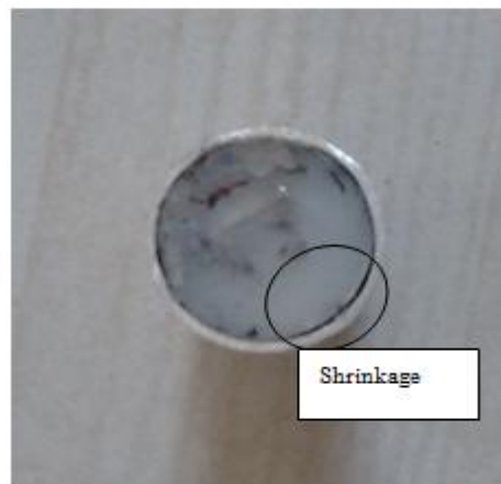
Fig.4. Shrinkage gap between Al6061 and PP
