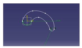
In sketcher we only draw the profile of the geometry. After drawing complete profile we need to check whether our profile is completely constrained or not.
