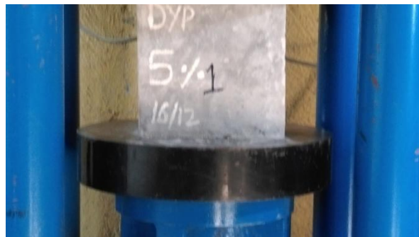
Photograph 1: Compressive testing of concrete block
