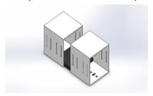
Fig: 8. two middle sections connected with a linker
