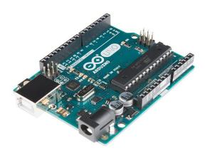
Fig: 10. Arduino board uno R3
