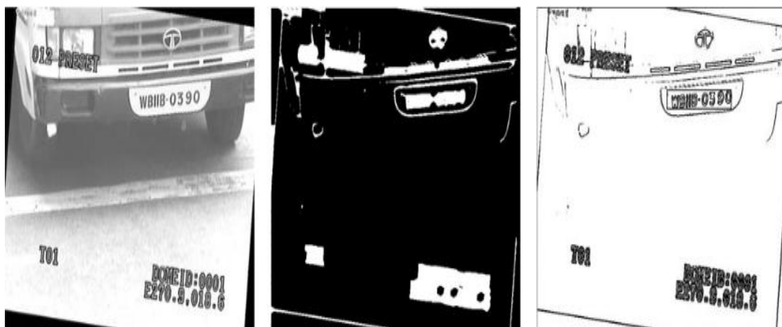
Fig.9: Segmentation result of automatic number plate recognition
