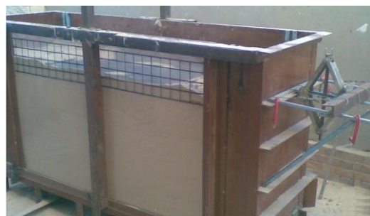
Fig. 3 Sand container and lateral stressing mechanism
