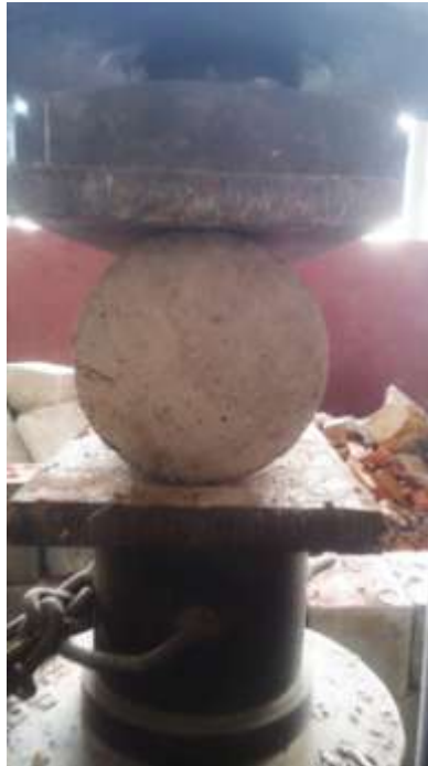
Figure 2- Specimen under Split Tensile Test
