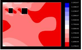
Figure 11. Von Mises Stress Plot of Steel Plate with Rectangular Cut-Outs 400 mm apart
