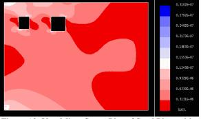
Figure 10. Von Mises Stress Plot of Steel Plate with Rectangular Cut-Outs 300 mm apart
