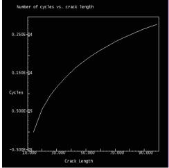
Figure 8. Crack length Vs No. of Cycles plot of Steel Plate with Rectangular Cut-Outs 500 mm apart
