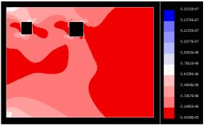
Figure 12. Von Mises Stress Plot of Steel Plate with Rectangular Cut-Outs 500 mm apart
