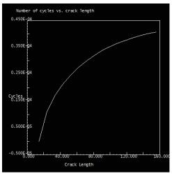
Figure 7. Crack length Vs No. of Cycles plot of Steel Plate with Rectangular Cut-Outs 400 mm apart
