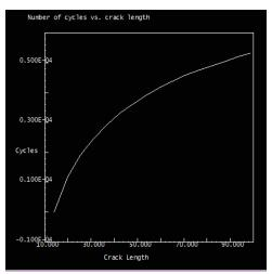
Figure 5. Crack length Vs No. of Cycles plot of Steel Plate with Rectangular Cut-Outs 200 mm apart
