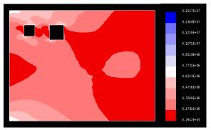
Figure 9. Von Mises Stress Plot of Steel Plate with Rectangular Cut-Outs 200 mm apart
