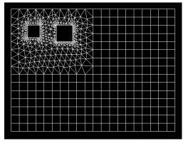
Figure 1. Finite Element Mesh of Steel Plate
