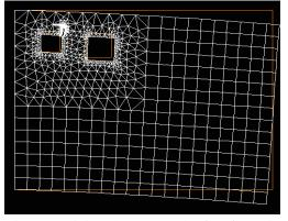
Figure 4. Finite Element Mesh of Deformed Shape after Crack Propagation
