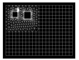
Figure 3. Finite Element Mesh of Crack at Corner of Cut-Out
