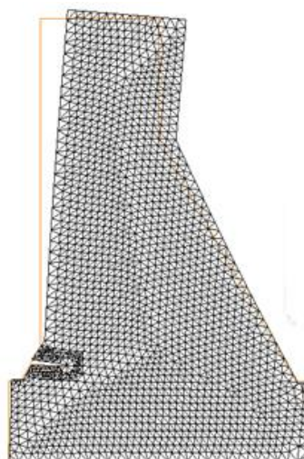
Fig. 2.2. Deformed mesh of the fem dam profile after application of the crack for the water level at the one third height of the dam height.
