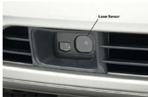
Fig.4 The Lexus LS430 laser sensor built into the front grille
