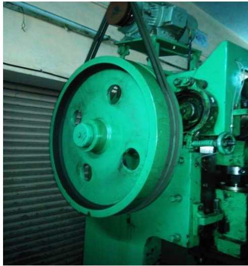
Fig.2. Existing Flywheel of machine
