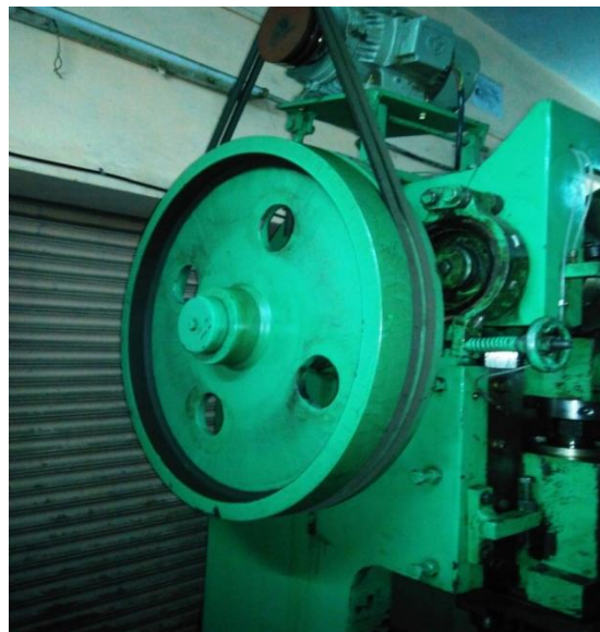
Fig.2. Existing Flywheel of machine
