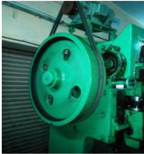
Fig.2. Existing Flywheel of machine
