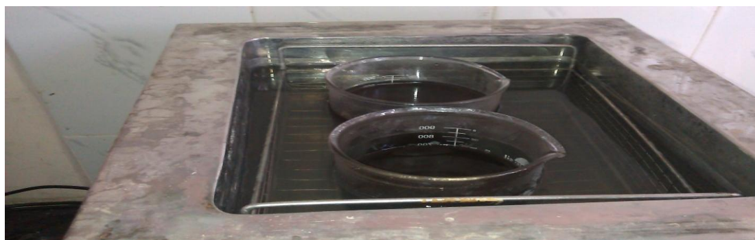
Figure 3: Ultrasonic Cleaner apparatus for sonication process of CuO Nanofluids
