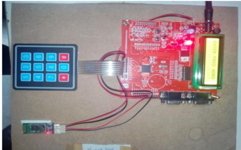
Fig4: The overview of system interface with controller, keypad and Bluetooth
