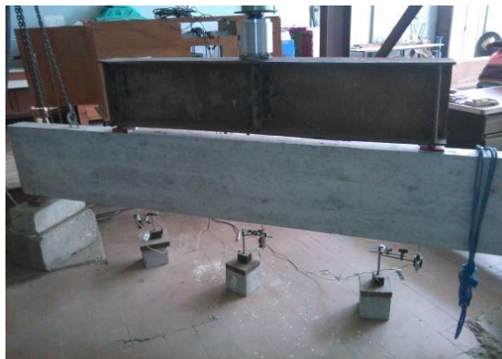
Fig (15): Testing of Shear Beam (SR5)
