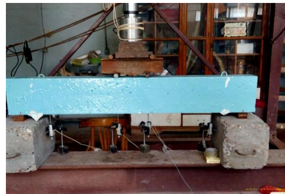
Fig (16): Testing of Flexure Beam (F3)
