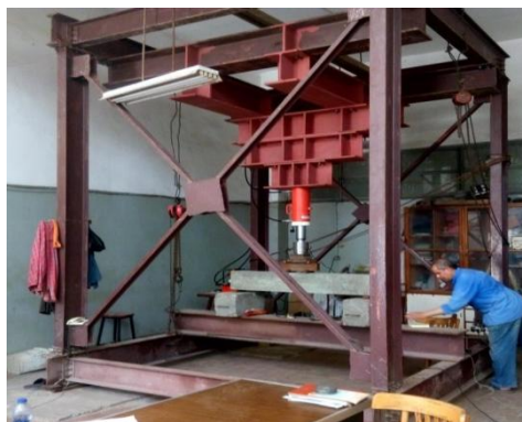
Fig (10): Frame Used in Testing Beams
