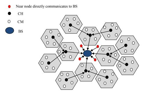
Fig. 3 MHCD-LEACH with direct Communication to the BS by Near Nodes
