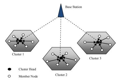
Fig. 1 Singlehop Communication for Small Network in LEACH
