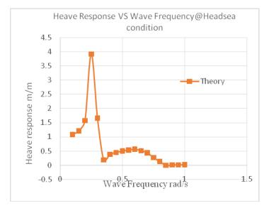
Figure 2: Heave RAO Semisubmersible Hull –Theoretical Calculation
