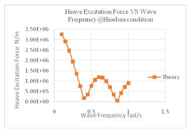
Figure 1: Heave Excitation Force Semisubmersible Hull
