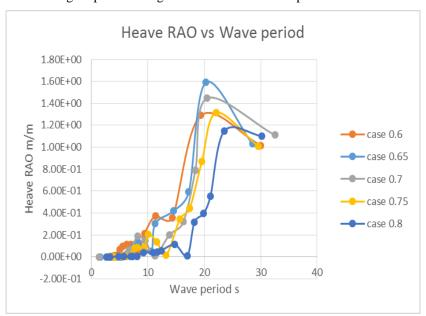
**Figure 8 Heave RAO for Different Volume Fraction**
