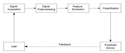
Figure 1: Block Diagram of a BCI System.
