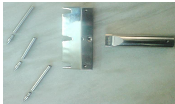
(b) Components of Yaw meter
