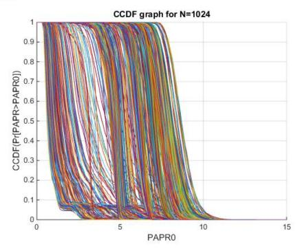
Figure-6: Figure shows variations in PAPR with different phase sequences obtained from the Riemann Matrix. The Minimum PAPR is achieved using the 1012th row of the Riemann matrix in this case.
