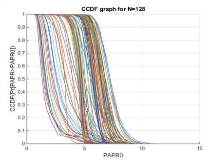
Figure-4: Figure shows variations in PAPR with different phase sequences obtained from the Riemann Matrix. The Minimum PAPR is achieved using the 1200th row of the Riemann matrix in this case.
