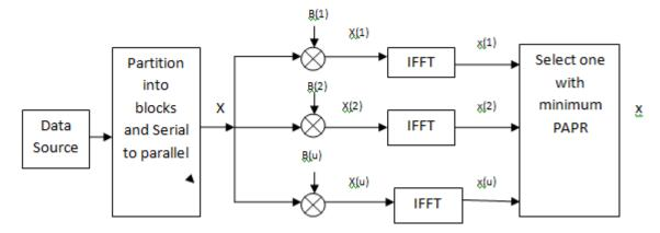
Fig. 1 Block Diagram of SLM
