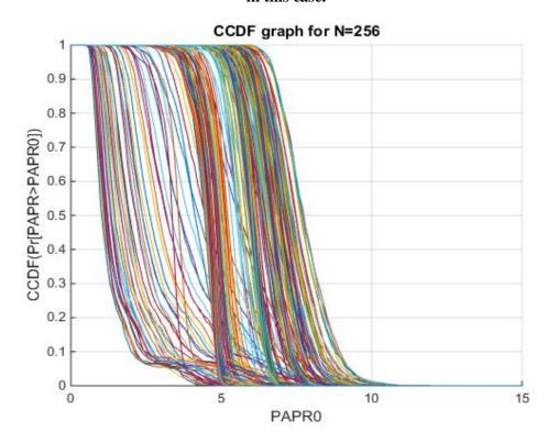
Figure-5: Figure shows variations in PAPR with different phase sequences obtained from the Riemann Matrix. The Minimum PAPR is achieved using the 240th row of the Riemann matrix in this case.
