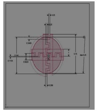
Fig 1: Meta Material Based Micro Strip Patch Antenna Designed Using Sonnet Lite Simulator
