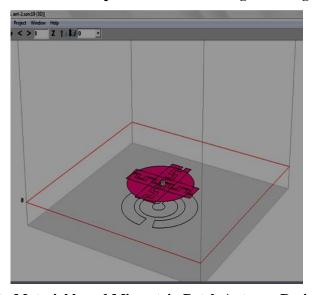
Fig.2: 3D View of Meta Material based Microstrip Patch Antenna Designed Using Sonnet Lite
