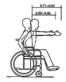
Fig.4 Horizontal Reaching Zones For Wheelchair User (All dimensions are in m)[5]
