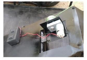
Fig.12 DC Motor and Switch Assembly
