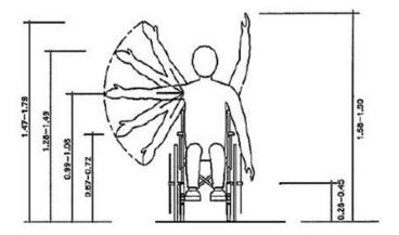
Fig.3 Vertical Reaching Zones of Wheelchair User (All dimensions are in m)[5]
