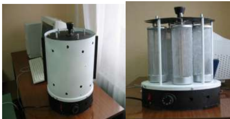
Fig.1. Infrared, Ecological, Universal, Portable Dryer Based on Indirect Application of Electricity As The Heat Source
