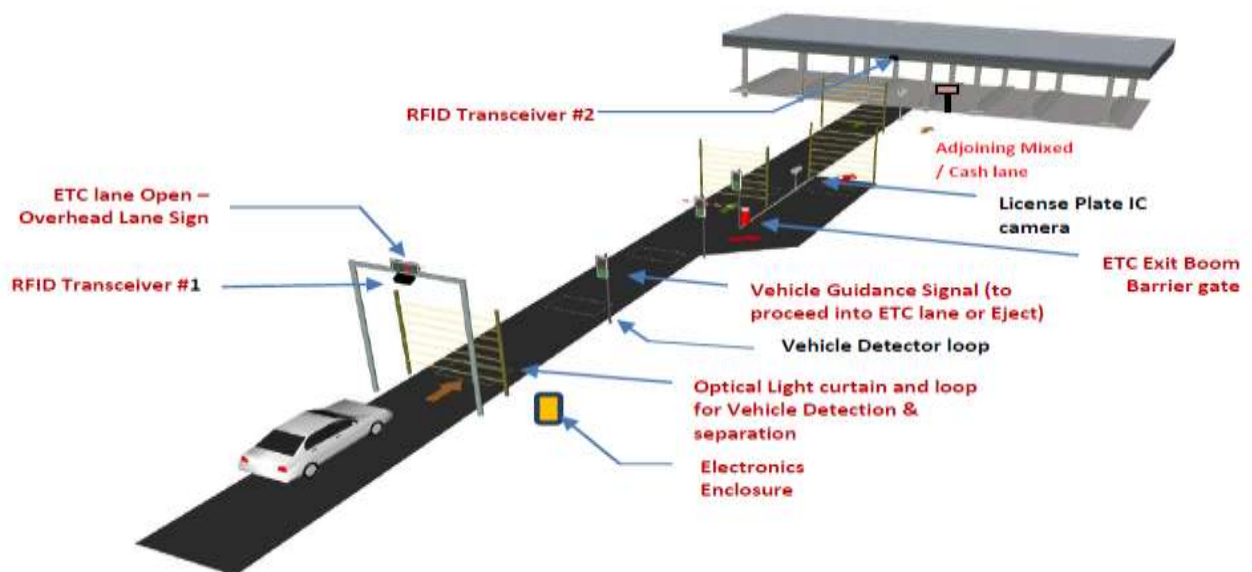
Fig. 1. General arrangement of ETC lane
