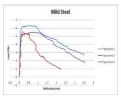
c) Load Deflection Curve for Steel Fibres Mix
