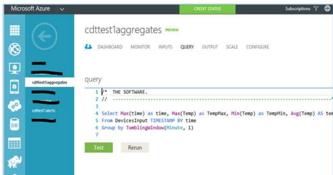
Fig. 13: Query run at Azure streamline Analytics to get real time data of temperature from Signal post module
