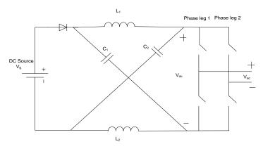
Fig. 2: H bridge (single phase) Z source inverter
