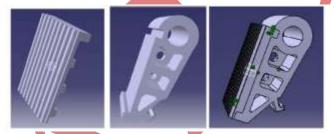
Fig 5: Assembly of swinging jaw plate with pitman
