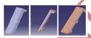
Fig 4: Sketching of swinging jaw plate with one, two and three stiffeners
