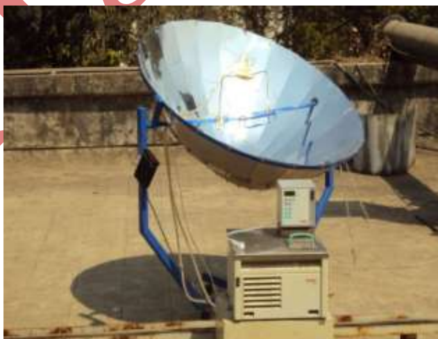
Figure 2: Experimental setup of photocatalytic degradation of meta-chlorophenol using solar radiations.
