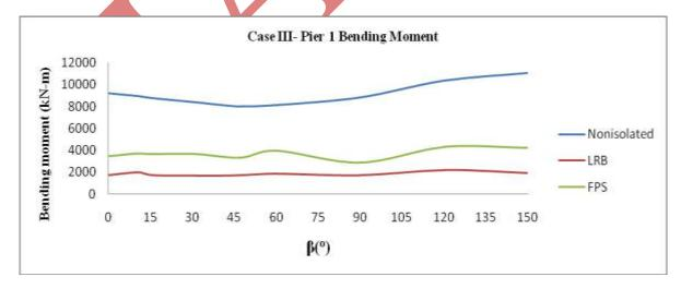
Fig.14. Case III-Pier 1 Bending Moment of Curved Bridges
