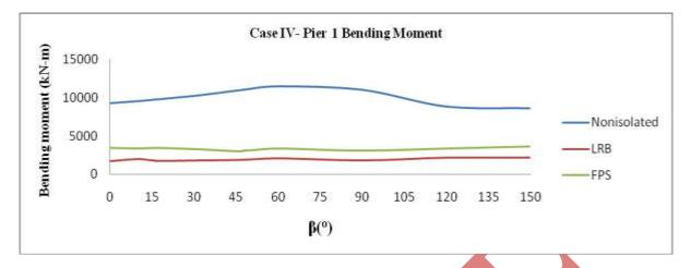
Fig.15. Case IV-Pier 1 Bending Moment of Curved Bridges
