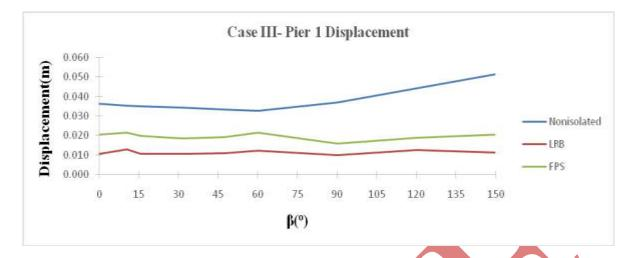
Fig.6. Case III- Pier 1 Displacement of Curved Bridges
