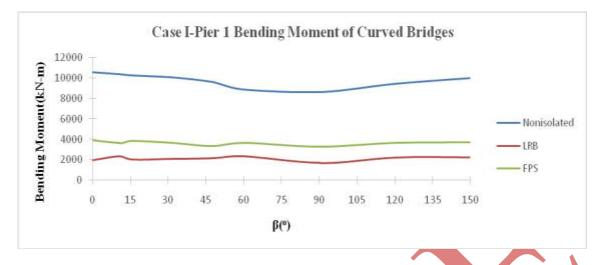
Fig. 12. Case I-Pier 1 Bending Moment of Curved Bridges
