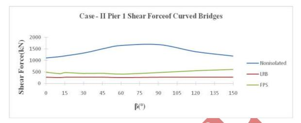
Fig. 9. Case II- Pier 1 Shear Force of Curved Bridges
