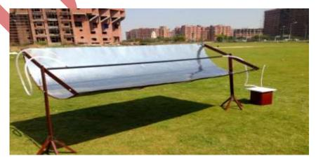
Fig. 1b: Working set up of Solar thermal Syphon Pump at Sharda University Greater Noida campus.
