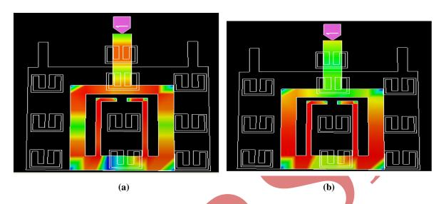
Fig.2. Simulated current distributions on the patch and ground plane, respectively, at (a) first notch frequency and (b) second notch frequency.
