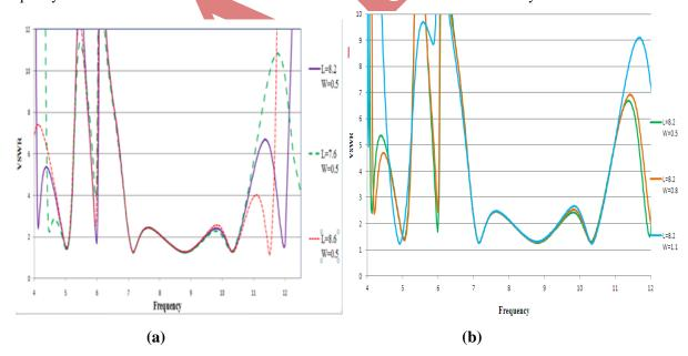
$Fig. \ 3 (a) \ Simulated \ VSWRs \ of \ proposed \ antenna \ with \ different \ length \ of \ L-shaped \ stubs$
