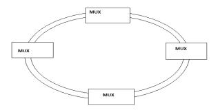
In this network structure, connections between network elements are bi-directional. The overall capacity of the network can be split up for several paths each with one bi-directional working line, while for unidirectional rings, an entire virtual ring is required for each path. If a fault occurs between neighbouring elements A and B, network element B triggers protection switching and controls network element A by means of the K1 and K2 bytes in the SOH.
