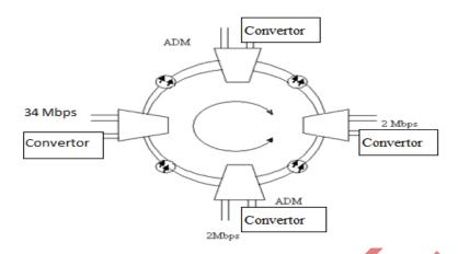
This purposed method is very convenient for the maintenance engineer. As he entered in the office he can see convertor to check the fibre cable faults. When the convertor shows the far end loss of particular station the fault location can be measured with help of OTDR and the action can be taken immediately. The following graph shows the distance for a particular fibre with the help of OTDR.
