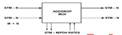
Having introduced you to the concept of an SDH Network, lets now take a look at the network "building blocks" and how they are configured. These network elements are now all defined in CCITT standards and provide multiplexing or switching functions.
