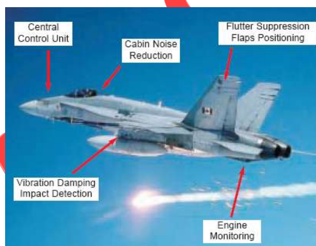
Fig. 3 Locations of Potential Smart Systems in an Aircraft [3]
