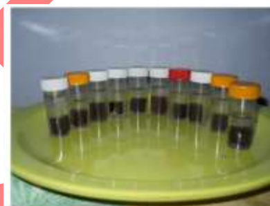
Fig.2.4 samples in water for water absorption test
